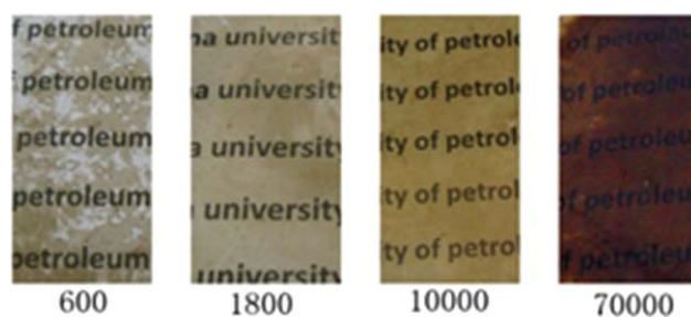
Figure 7. Transparency of PEI/GO composite films prepared from PEIs with different molecular weights. [Color figure can be viewed in the online issue, which is available at wileyonlinelibrary.com .]
