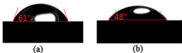
Figure 3. Water contact angle of the membrane for: (a) untreated film, and (b) treated film. [Color figure can be viewed in the online issue, which is available at wileyonlinelibrary.com.]
